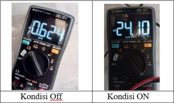
Picture 19. Tension Test Results with Avometer
